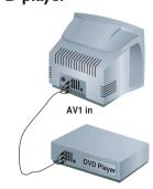
■ Connect the TV's green, blue and red Y Pb Pr (AV1 in) jacks to the corresponding COMPONENT VIDEO OUT jacks on the
